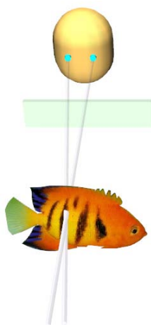
Fig. 1. Our virtual robot, Emer. His name is based on “emergent”, our neural network simulator. Seen here are his torso, head, eyes, eye-beams, and the fish that he is foveating in preparation for object recognition. Emer is implemented using the Open Dynamics Engine rigid body physics simulator [6] and the Coin3D 3D Graphics Developer Kit [4]. Each of his eyes is a camera, and their offset positions on his head give him slightly different views of objects, facilitating stereo vision.
